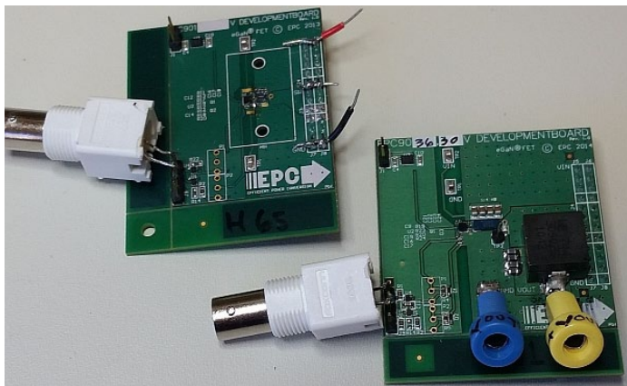
Figure 1 The test boards are shown with the half bridge configuration only on the left and the complete DC/DC converter on the right. The banana sockets allow connection of the board to an electronic load. BNC connectors provide access to an external pulse generator.
